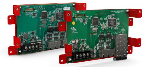
Ethernet and Fiber cards are interoperable and both types can be used within a network. When using fiber, both single mode or multi mode can be utilized, matching a building's existing infrastructure.
