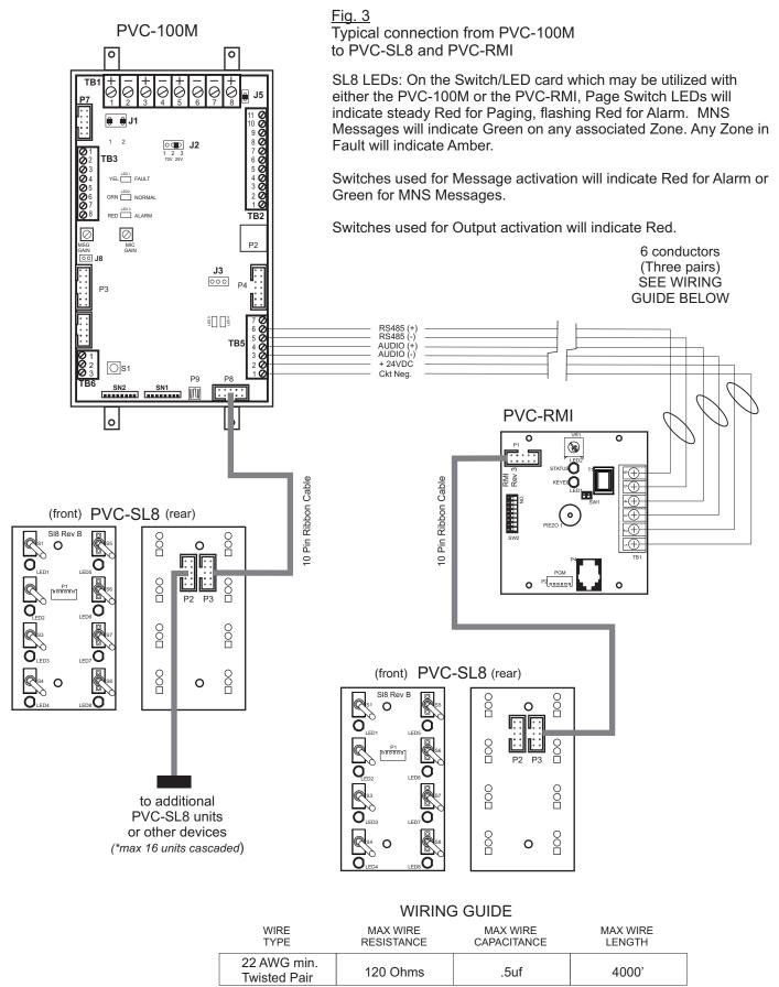
Wire for 24 VDC pair must be sized to insure no more than a 20% drop in voltage at the last device
