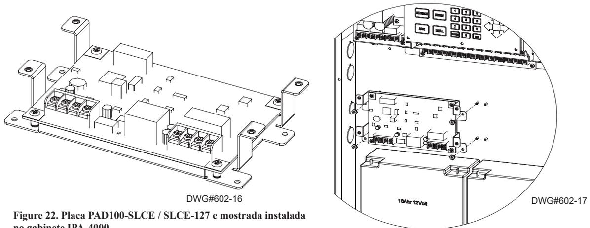
Figure 22. Placa PAD100-SLCE / SLCE-127 e mostrada instalada no gabinete IPA-4000
