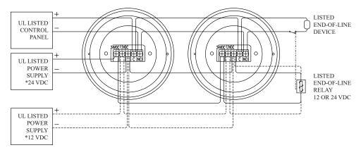
\* USE EITHER 12 VDC OR 24 VDC. THEY CANNOT BE USED SIMULTANEOUSLY.
