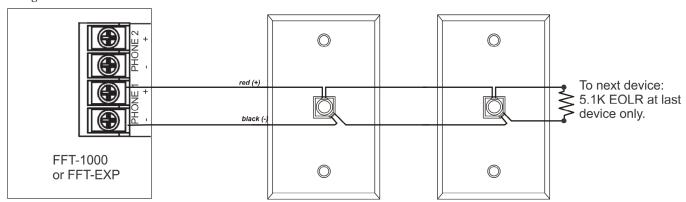
Class A Wiring Connection
