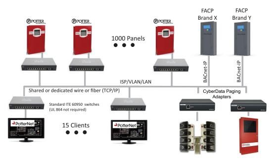
*Note:* UL 864 systems require UL approved computer and monitor from Potter. IT equipment (switches/routers/etc) do not need to be UL 864 listed but must have standard ITE 60950 listing.
