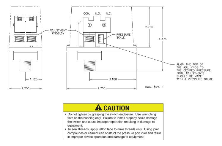
**MOUNTING:** Device should be mounted in upright position. (Threaded connection down.)
