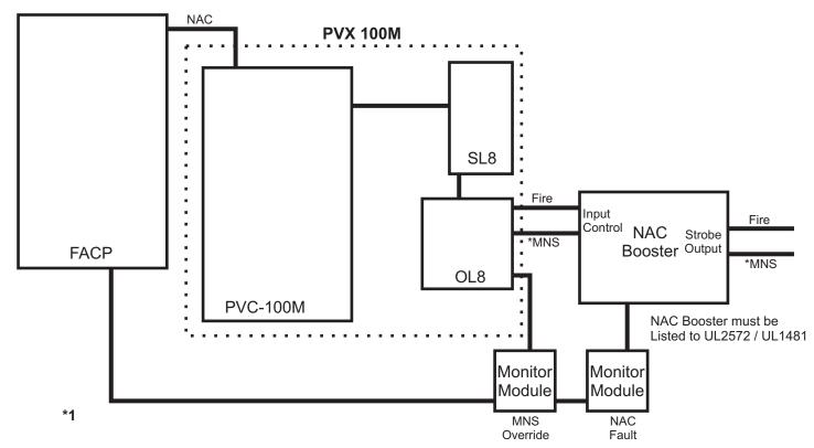
The PVX 100M may be used in conjunction with a UL Listed FACP. The FACP must be capable of monitoring contacts for Fault conditions and Supervisory conditions in order to report a MNS override.
