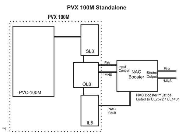
In applications where no automatic Fire Alarm initiation or notification is required, the PVX 100M may be used as a Standalone system. The PVC-IL8 will provide input points to monitor the Fault status of the NAC Booster.
