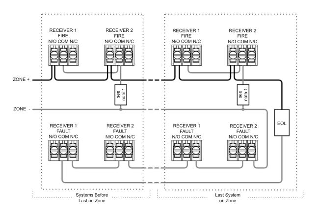
Note 1 - This component is the Fire Resistor. Its value is specified by the FCP manufacturer, and is not supplied with the System Controller. For U.S. installations it is typically a short circuit.
