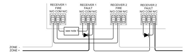
Single Receiver connected to Controller on "Receiver 1":
