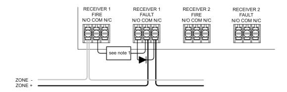
Note 1 - This component is the Fire Resistor. Its value is specified by the FCP manufacturer, and is not supplied with the System Controller. For U.S. installations it is typically a short circuit.
